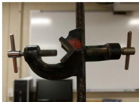
Figure 2: Double-ended bosshead clamp
