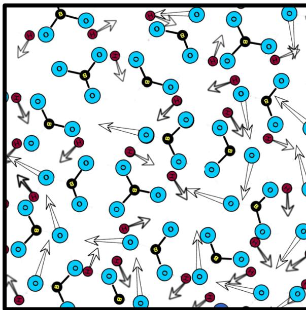
Figure 11: With the addition of heat, bonds between the hydrogen and some oxygen break, forcing the hydrogen and oxygen to move around. Boroxol rings and trigonal borate are freed to move around.
