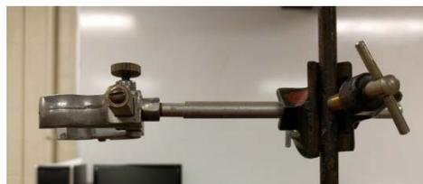
Figure 3: Extension clamp (slide-ended)
