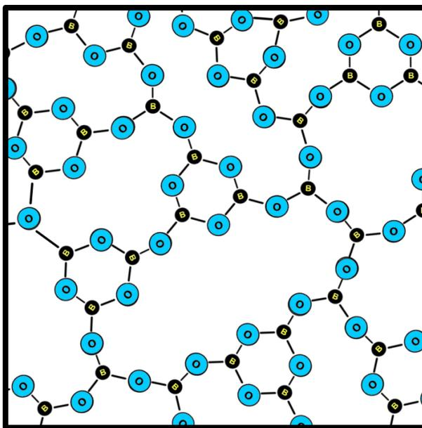
Figure 13: All the water has now evaporated and the borate glass has fully formed. Note the presence of both boroxol rings and trigonal borate in the network.
