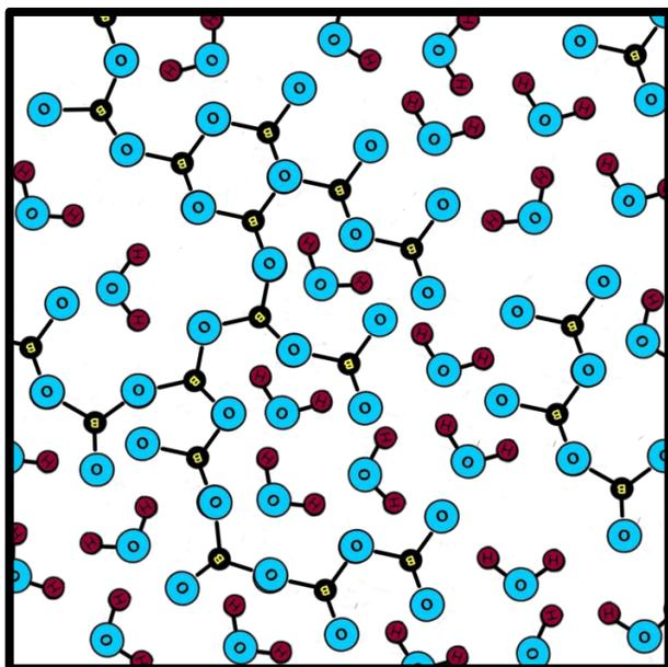
Figure 12: All hydrogen will bond in pairs to free oxygens, creating water molecules, while the trigonal borate and boroxol rings bond to one another forming the final glass network.
