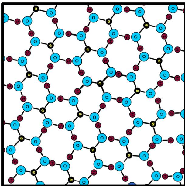
Figure 10: The  $H_3BO_3$  structure before heating. All molecules are stably bonded and immobile.
