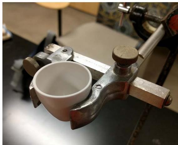
Figure 4: Mounted ceramic crucible.
