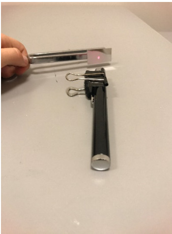
Figure 3 Keeping the laser pointer on with a binder clip, hit the tuning fork to set into vibration, and move it up and down to observe the sine waves off the laser's reflection. Image will be on the wall to the right of this setup.
