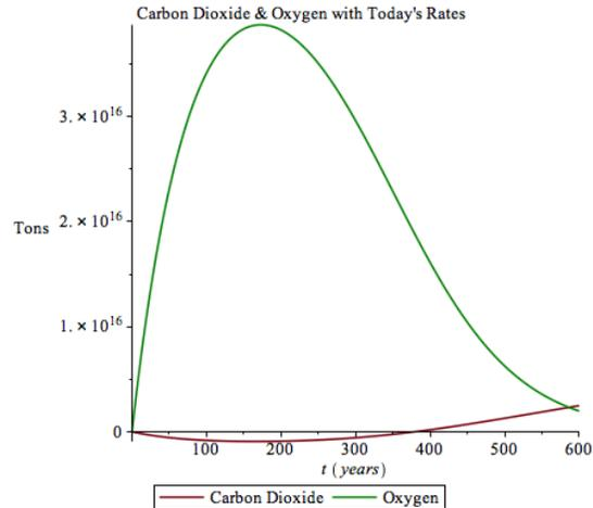
**FIG. 2.** The model's atmospheric carbon dioxide and oxygen abundances,  $C(t) - C_0$  and  $O(t) - O_0$ , using rate coefficients held at their 2018 values.  $t = 0$  denotes the year 1500.
