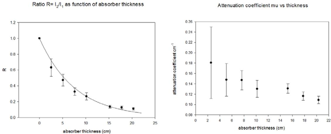
**FIGURE 3.** Left: Transmitted over incident flux vs. absorber thickness. Right: Absorption coefficient  $\mu$  vs. absorber thickness.
