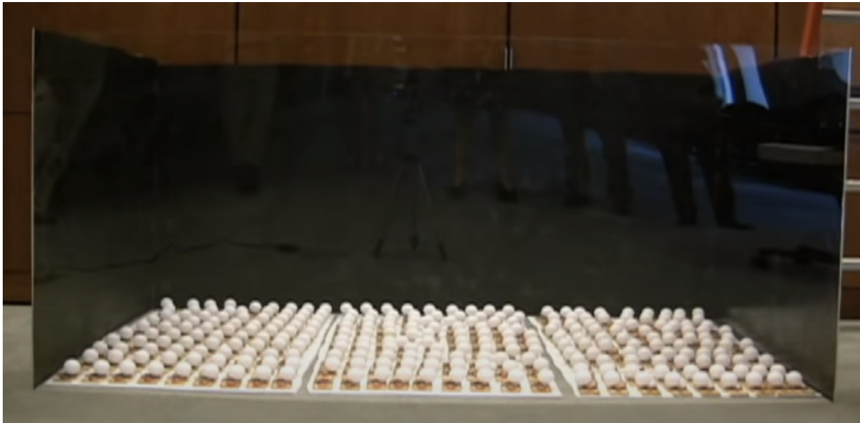
Figure 2: a full array of ping pong balls set on armed mousetraps
