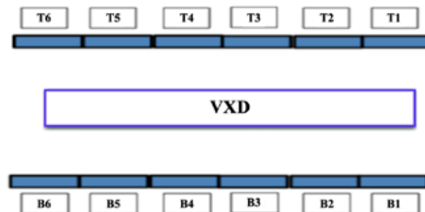
FIGURE 1. A schematic of the VXD cosmic trigger system with six top and six bottom scintillators.
