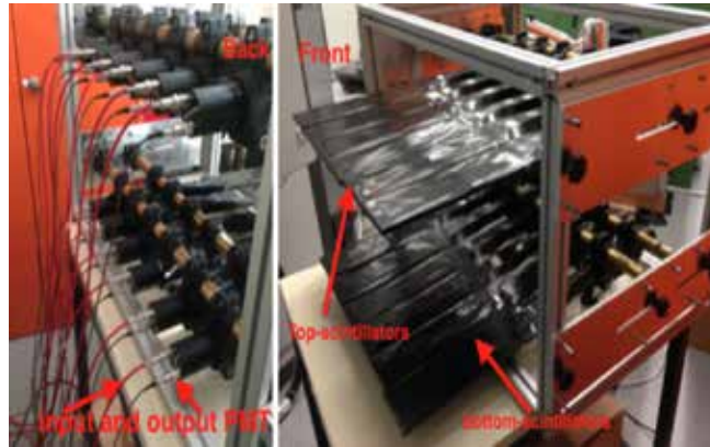
FIGURE 4. All scintillators, with PMTs, are Installed in the frame, and tested.
