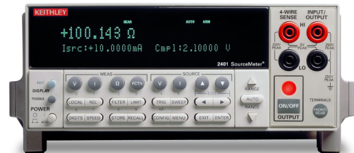
Figure [2]; The Keithley 2400 SMU unit
