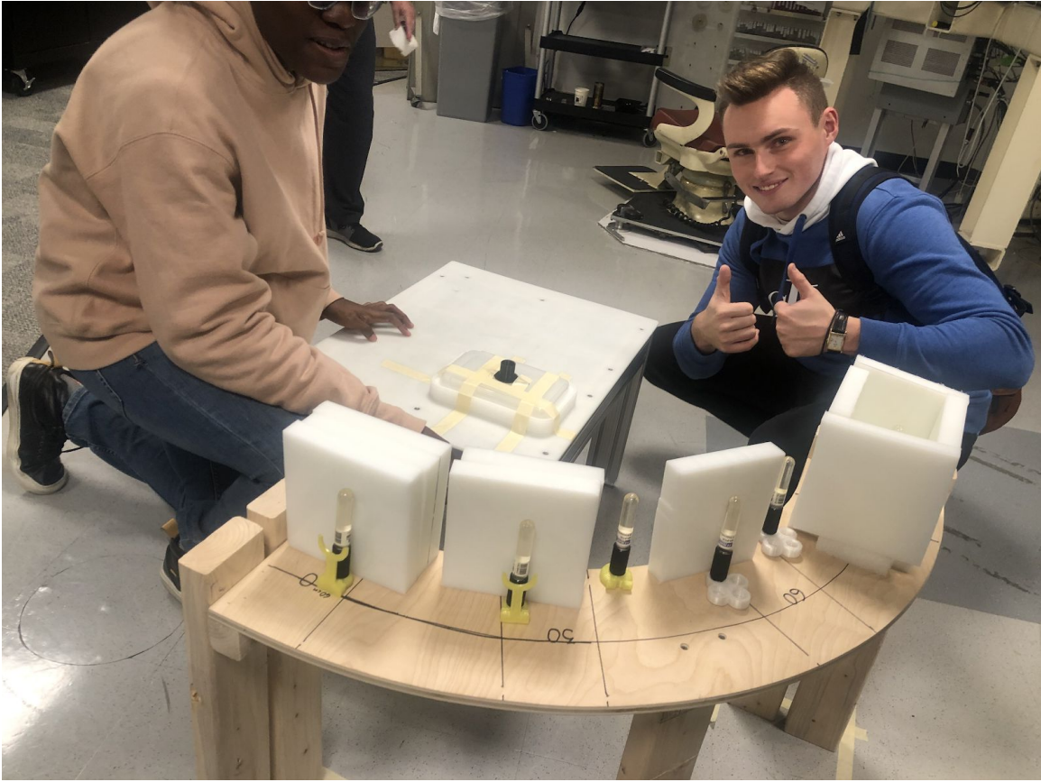
Students with the bubble detector and shielding set up
