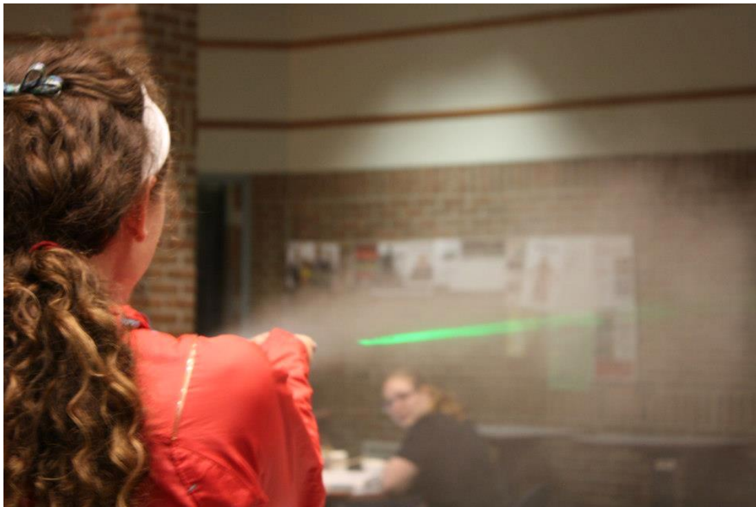
IWU-SPS Secretary Amanda Wolfe shows how a laser beam scatters off aerosol particles to create a visible beam.
