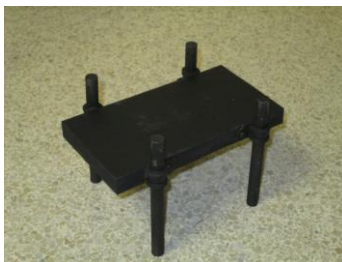
Figure 2: Bench-tripod adapter used to connect the optics bench to a tripod.
