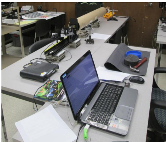
Figure 3: The optics bench rests on lab jacks and is aligned with a light source at the opposite end of a long tube. The sensors (light sensor and rotary motion sensor) are connected to the laptop running DataStudio software.
