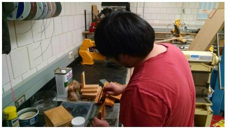
Left: Senior Ivan Tso applies the water seal to each mold piece before construction. The molds had to be weather resistant due to the amount of ice and melted snow that they are exposed to, and once connected the molds were sanded for safety purposes.
