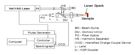
Figure 1: Experimental set-up to obtain the LIBS spectra.
