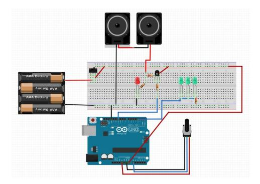
The diagram above describes the set-up. A Potentiometer resistor will provide input to the Arduino board and will function as our interface to tweak the frequency for the experiment. The current value will be shown to the user through a Seven Segment display (represented here as 3 green LED's). The Arduino will output the signal to the speaker using Pulse Width Modulation, which will be amplified by an NPN transistor connected to a 9v source.
