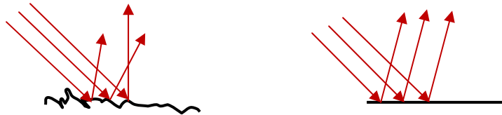
Figure 1: diffuse reflection (left) and specular reflection (right)
