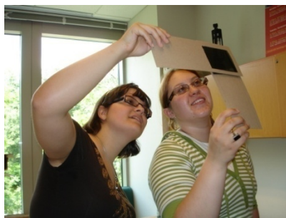
Figure 2: L: polarizers are parallel and light gets through. R: one is rotated 90°, blocking the light.
