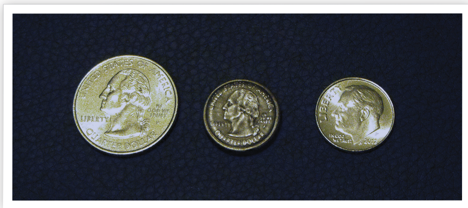
EXTREME CURRENTS pulsed into a small coil of wire shrank a quarter to the size of a dime. Photo by Niall O'Brien.
