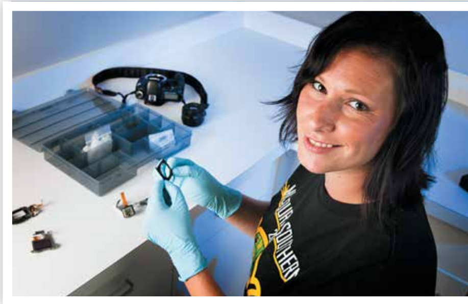
KRIS PRITCHARD holds a fixture that was 3-D printed to hold the magnesium fluoride radiator. Photo by Curtis Almeter.
