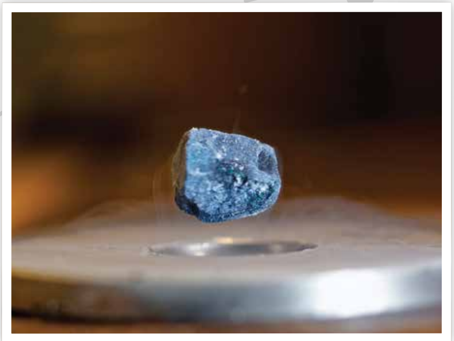
A MAGNET LEVITATES above a piece of superconductor cooled to -196^{\circ}\text{C} . Photo by Julien Bobroff, Frederic Bouquet, Jeffrey Quilliam, LPS, Orsay, France.
