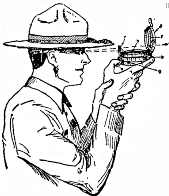
USING A MAGNETIC COMPASS. Photo courtesy of the United States government printing office.
