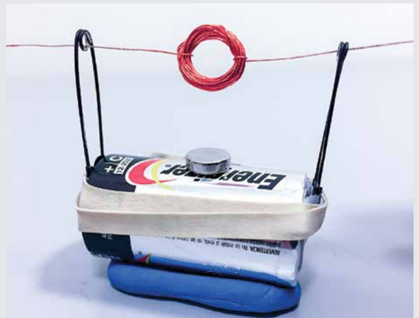
FIGURE 3: The fully assembled electric motor. Photos courtesy of Jacob Robertson and Zakary Noel, 2017 SPS SOCK interns.
