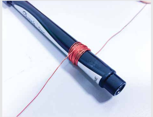
FIGURE 1: Wrap the coil around a circular object like a marker.
