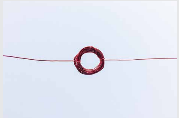
FIGURE 2: Slide the wire off the pen to create a coil. Diameter is ~1 cm.
