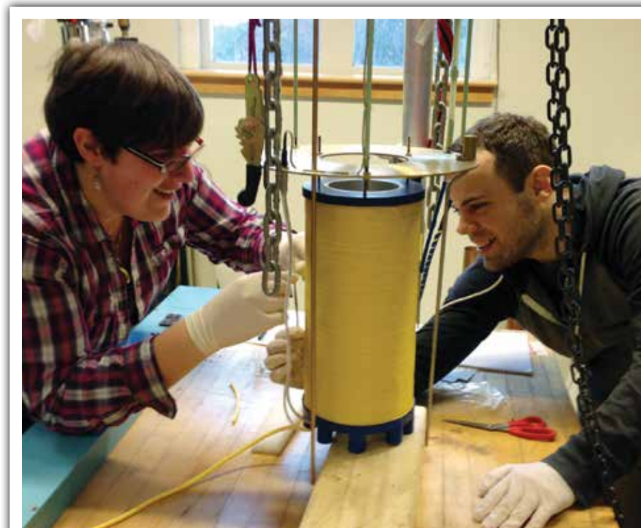
Dr. Long installing the solenoid for the University of New Hampshire's new DNP polarizer. Photo Courtesy of University of New Hampshire.
