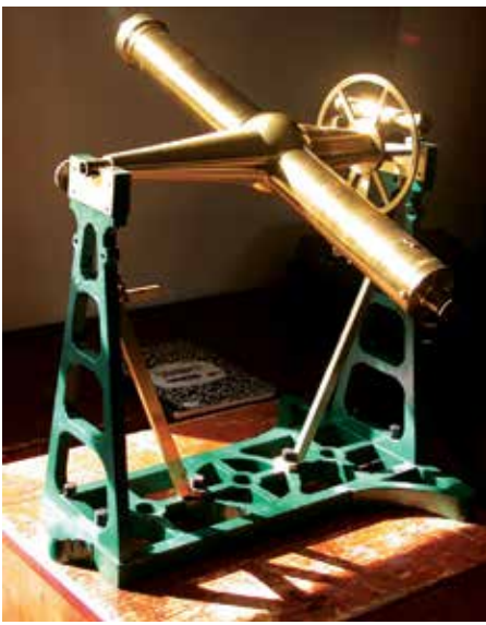
LEFT: The Parkinson & Frodsham transit instrument, Liverpool, circa 1838, from the Ladd Observatory history of science collection. Photo by Mike Umbricht / Ladd Observatory.
