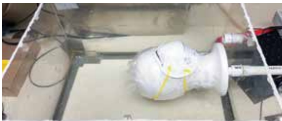
TOP: The view inside of Nazeeri's experiment, showing a head model outfitted with an N95 mask. Photo by Albert Nazeeri.
