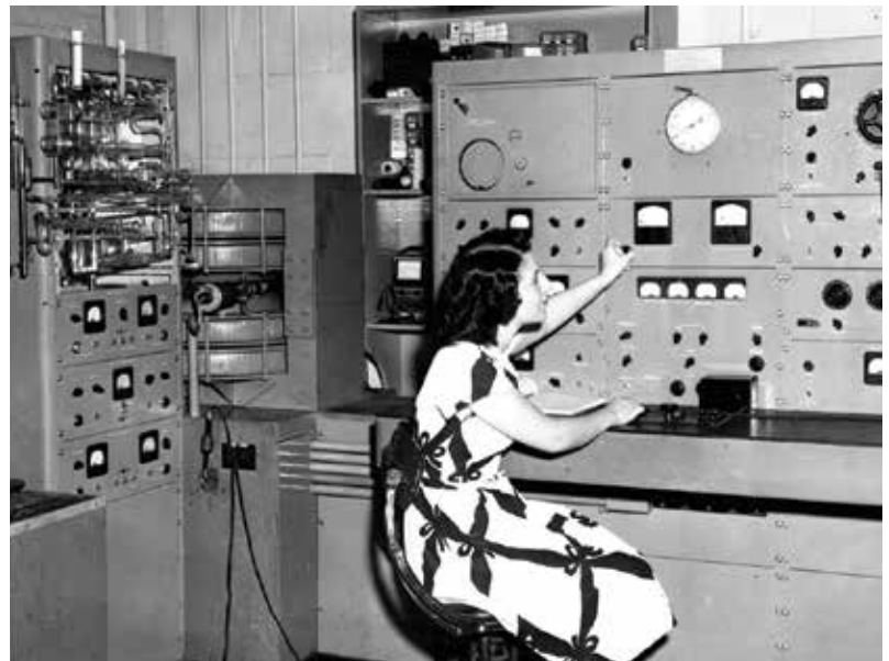
TOP: Photographs of a system that was developed for the Atomic Energy Commission designed to monitor radioactive fallout and used during the 1955 atomic bomb tests in Nevada. Left: Control station that includes a radiation monitoring switchboard (bottom), time-gates frequency counter (middle), and digital scanner (top) that supplies printing signals to the printer (right, next to switchboard). Upper right: Typical radiation monitoring station installation. Photo credit: National Institute of Standards and Technology, Gaithersburg, MD.
