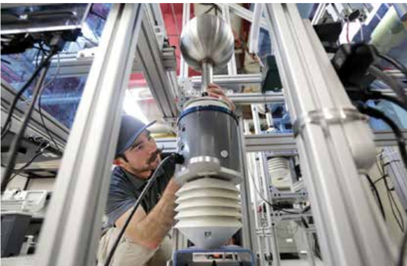
Understory field engineer Jonathan Mikolaiczuk tests one of the company's automatic weather stations. The silver ball at the top houses most of the sensors for all types of weather measurements including hail, rain, temperature and wind.
