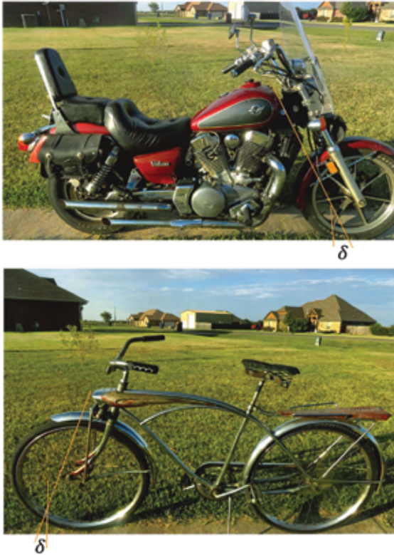
Figure 2: Showing the castor distance \delta on a 1994 Kawasaki Vulcan (top) and a 1962 J.C. Higgins Flightliner (bottom). Their front wheels have been deliberately set straight ahead. Photos by Dwight E. Neuenschwander.
