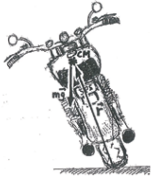
Figure 3: The torque produced by only the weight of the bike-rider center of mass (rider not shown) when leaning. The torque \mathbf{r} \times (m\mathbf{g}) points toward the back of the bike. All sketches by Dwight E. Neuenschwander.
