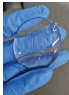
A sodium aluminosilicate glass sample Hauke synthesized. Photo courtesy of the author.
