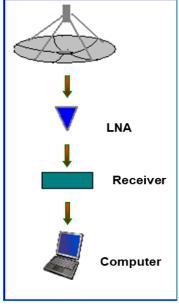
Figure 3 Radio telescope basic components [11].
