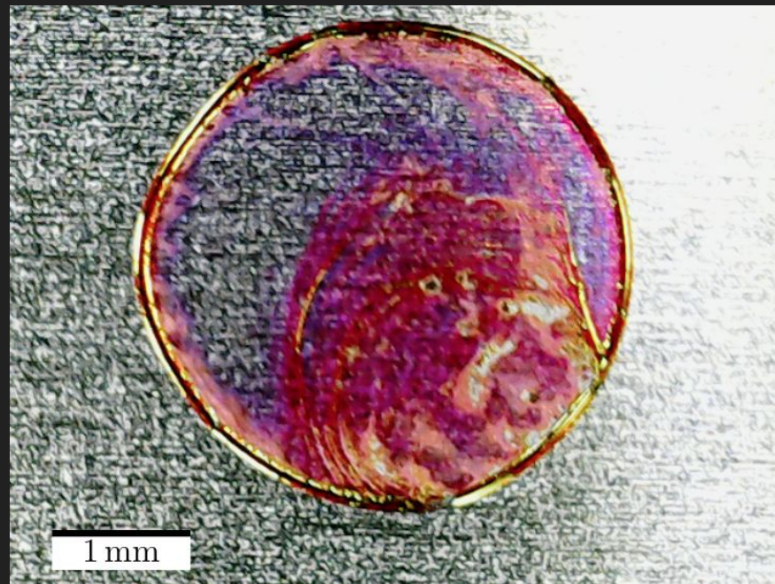
Figure 2: Deposition from a 0.5 microliter droplet with a rhodamine concentration of 0.49 mg/mL
